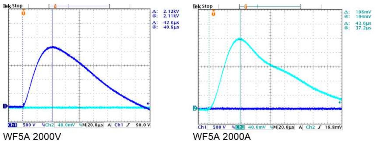
Figure 7: Hybrid coupler waveform open and short circuit for WF5A.
