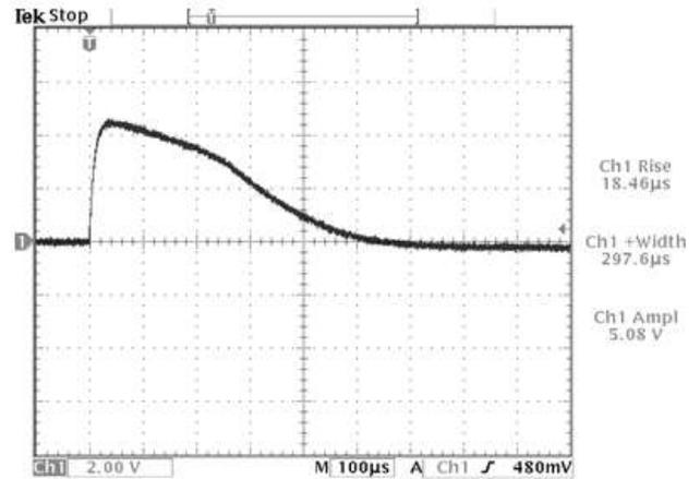
WF5B Iron core in saturation
