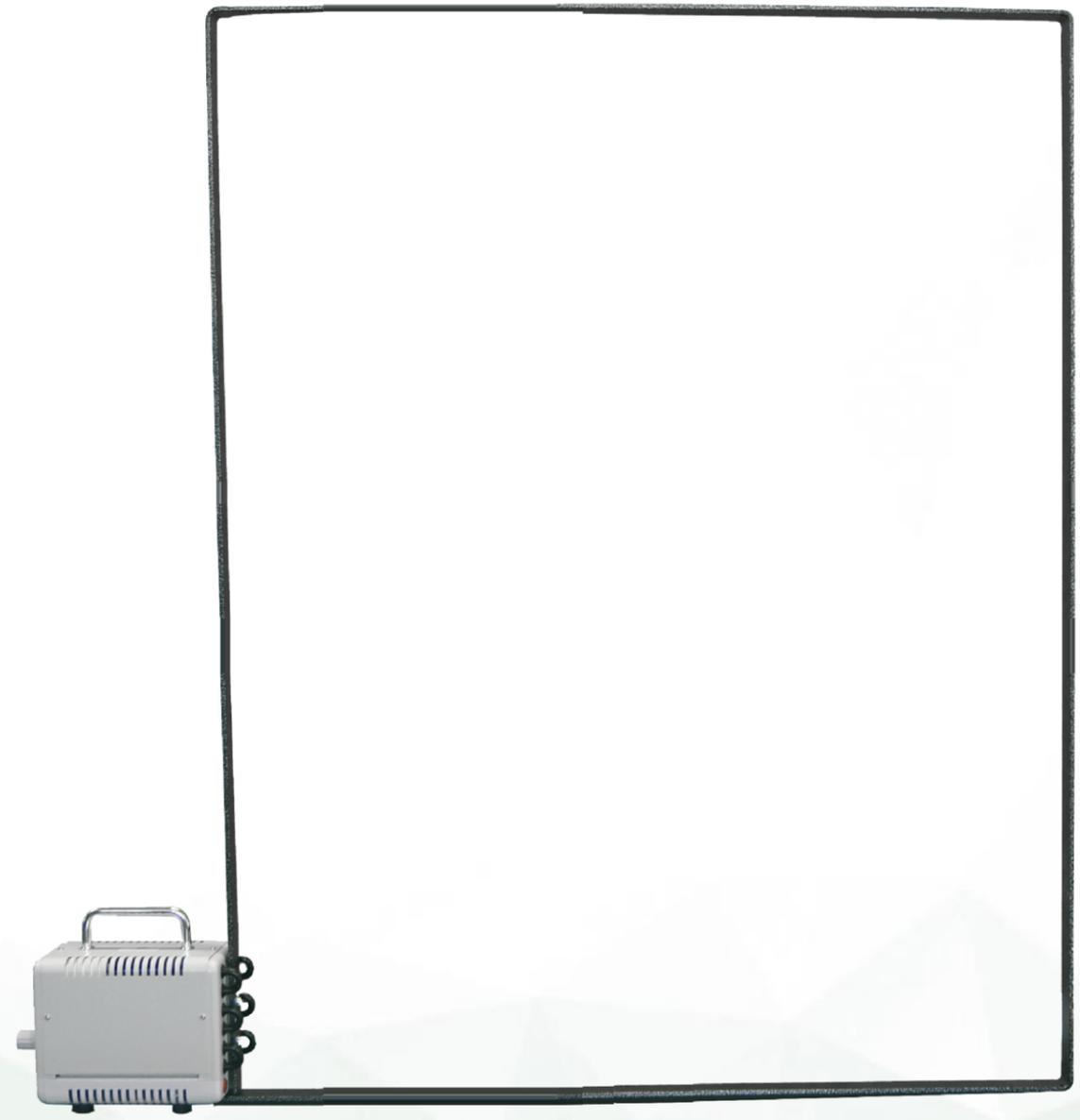
1.6.1. Magnetic pulse: IMU3000 S, MF1000-1, calibration setup
