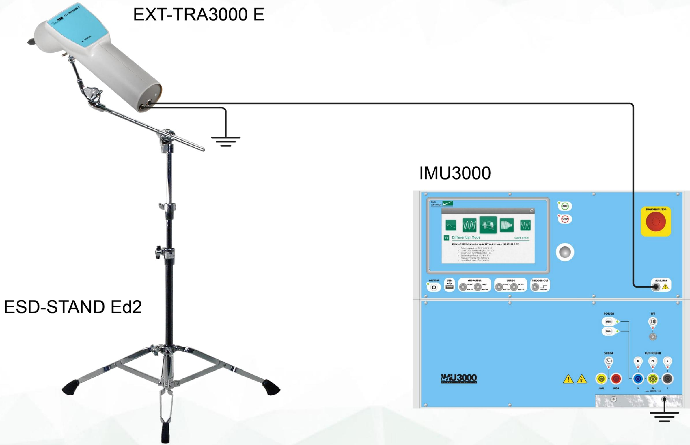
The stand is optional, recommended for tests that require many discharges in a fixed point of EUT.
