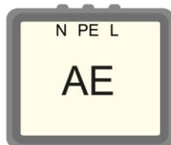
Auxiliary Equipment, could be single phase, three phase (when marked) or equipped with I/O ports
