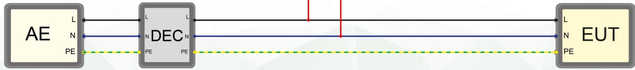
Decoupler could be a CDN like CDN2000-06-25. AE side could also be a supply.
