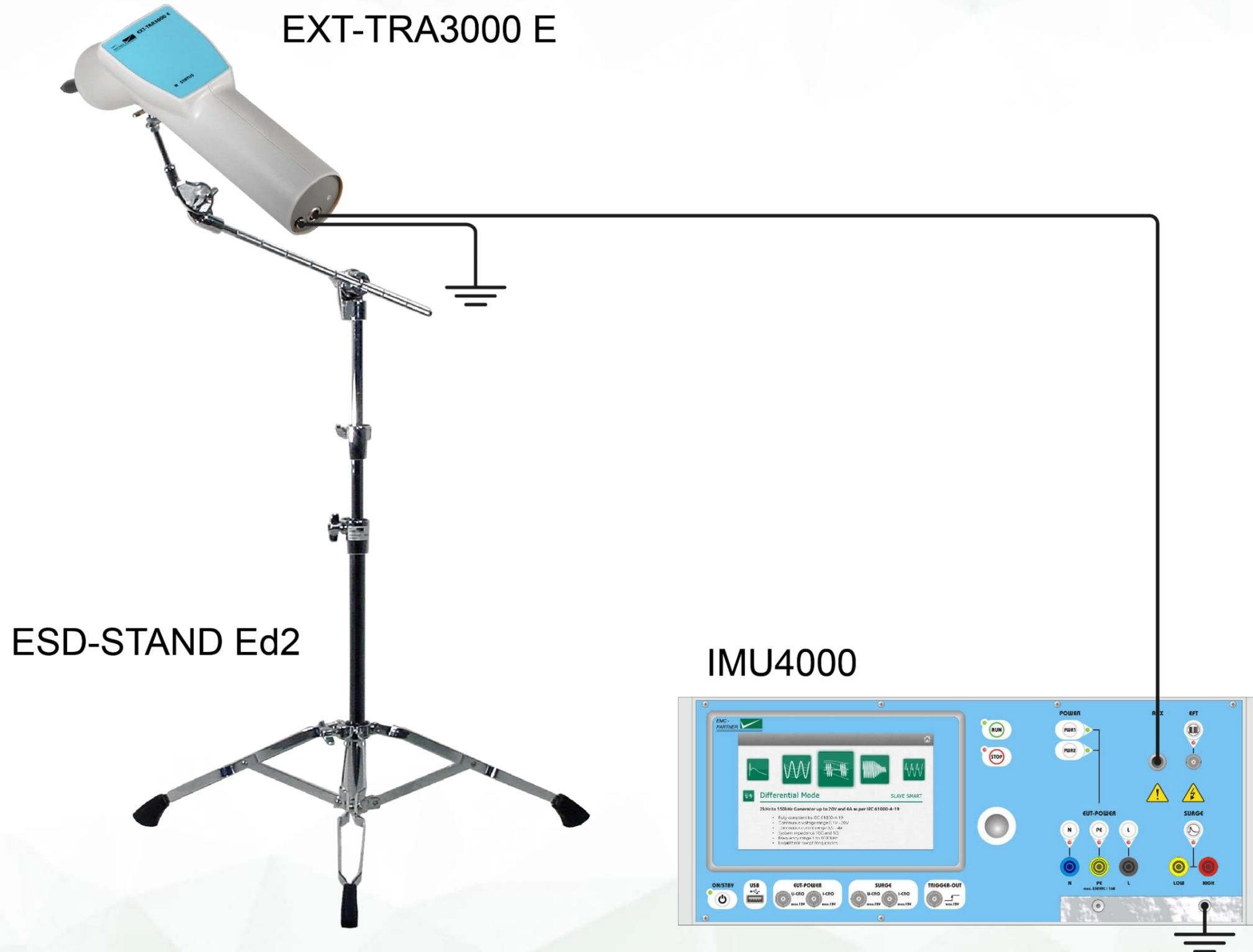
The stand is optional, recommended for tests that require many discharges in a fixed point of EUT.
