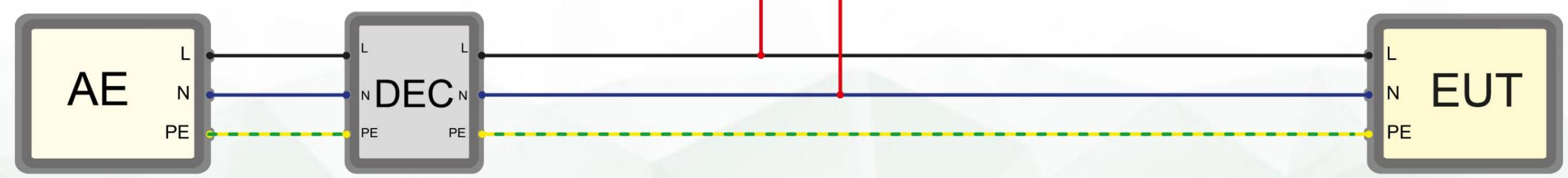
Decoupler could be a CDN like CDN2000-06-25. AE side could also be a supply.
