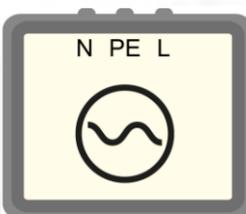
AC power source: could be grid connection or dedicated power source, one phase or three phase (when marked)
